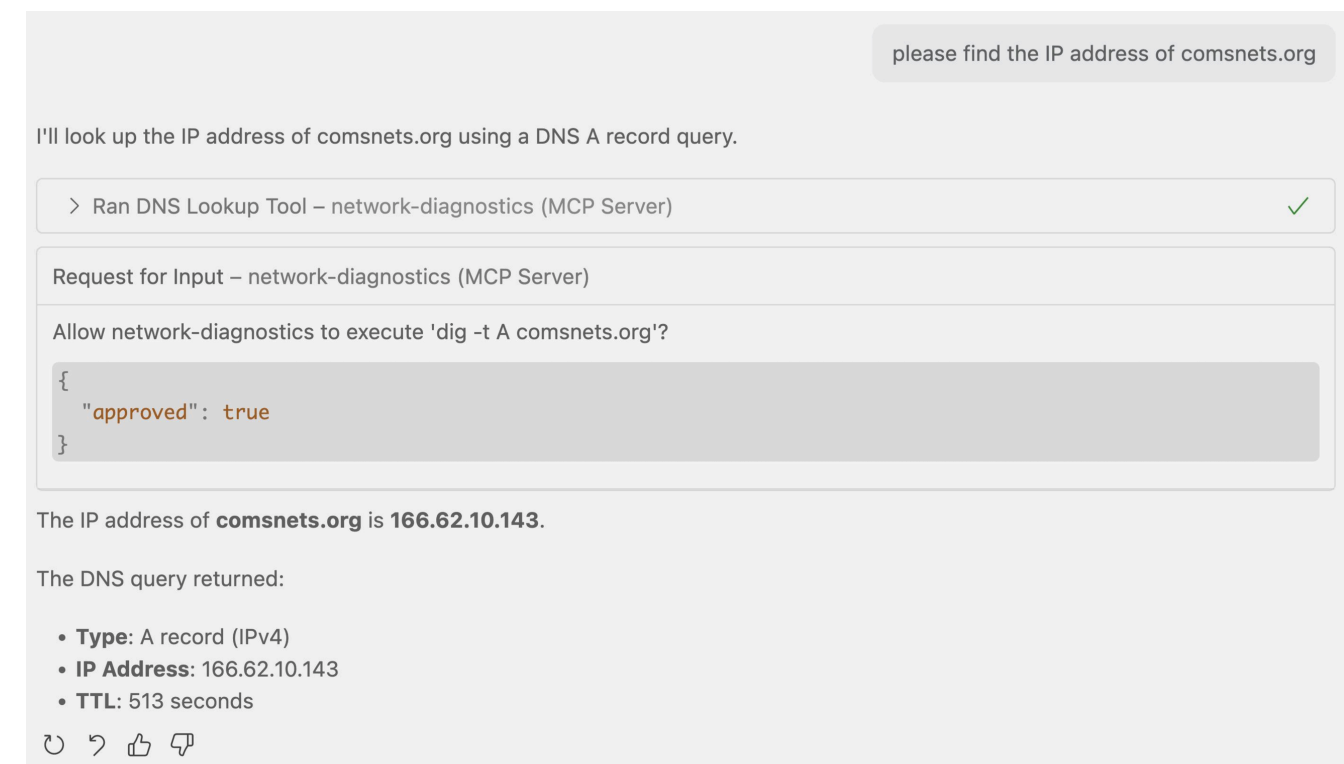
Figure 2: Validation via VS Code MCP Host. A single workflow demonstrating the architectural guarantees: (1) Interoperability: Running inside a standard third-party host. (2) Reasoning: The LLM inferred dig was required from a natural language query. (3) Elicitation: The protocol paused execution for user approval. (4) Synthesis: The agent received structured JSON, not raw text, enabling it to summarize the DNS record type and TTL accurately.
